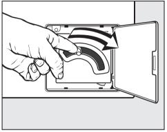
■ Push the emergency drain lever downwards (see illustration) and hold until no more water runs out.
