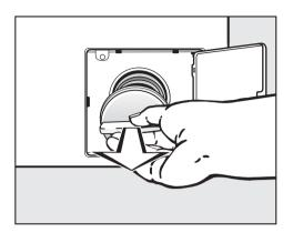
■ Remove the drain filter completely.
