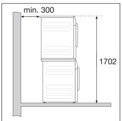
The washing machine can be installed as a washer-dryer stack together with a Miele tumble dryer. This requires a Miele washer-dryer stacking kit which can be purchased separately.
