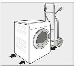
If transporting the washing machine with a sack truck, make sure its left or right side is resting on the truck.
