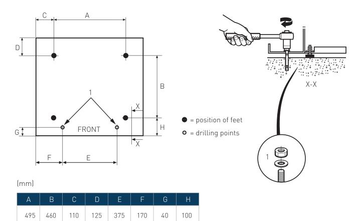
To ensure steadiness of the machine; the machine must be fastened to the floor. Place the machine over the two drilled holes. The holes are at the front of the machine. Level the machine with the feet of the machine. Screw in the feet as much as possible before starting to level the ma-chine. This will make the machine stand steadier. The maximum height adjustment of the feet is 30 mm.
