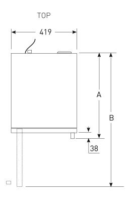
1. Electrical connection, 1.7 m cable with earthed plug included
