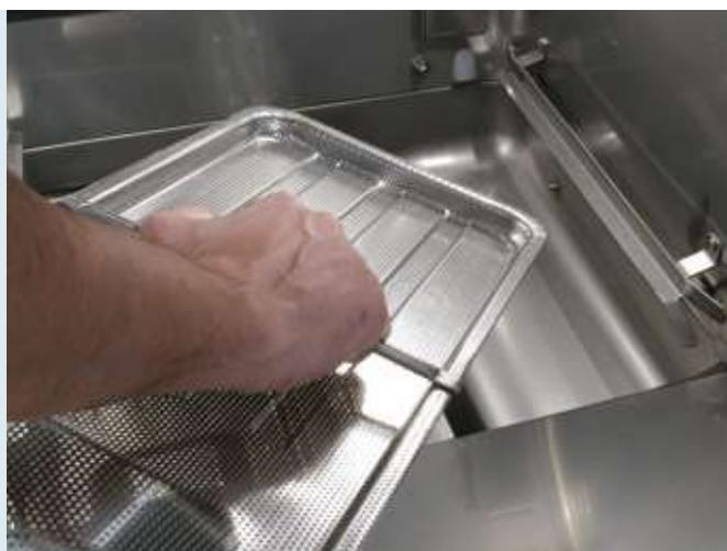
**Wash tank filters** can be **easily removed** without having to remove the washing and rinsing arms.
