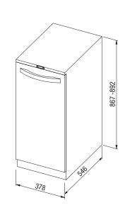
Depth is 610 mm with connected power cord. Front door handle sticks out an additional 45 mm.
